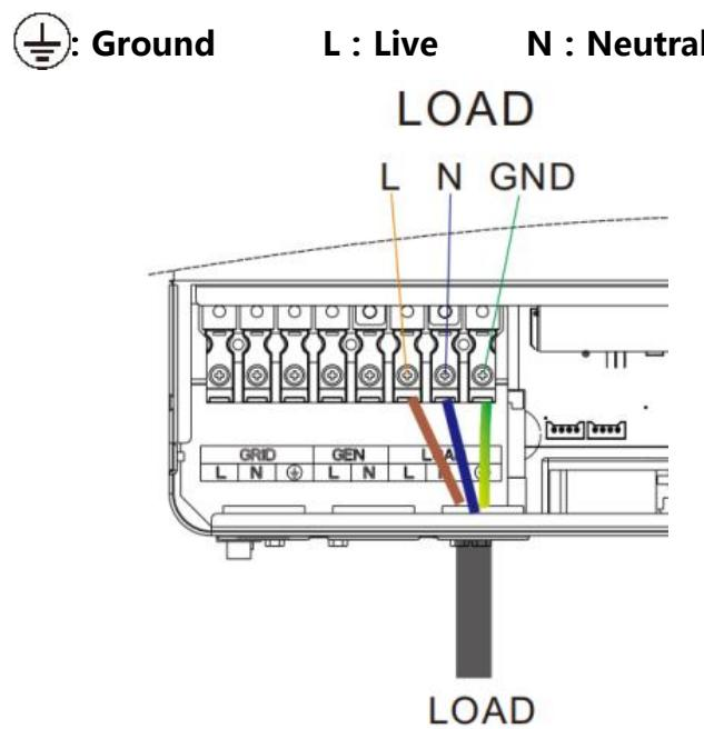
**Note:** The grounding wire shall be as thick as possible (cross-sectional area is not less than 4mm<sup>2</sup>). The grounding point shall be as close as possible to the all-in-one solar storage inverter. The shorter the grounding wire, the better.
