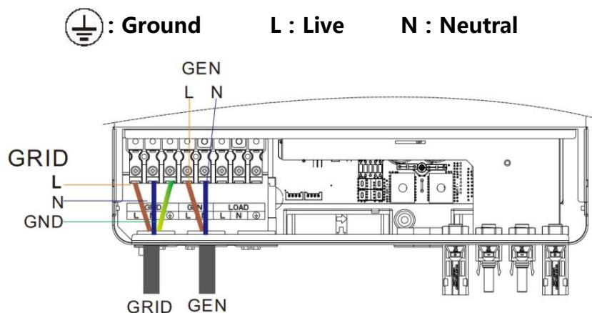
3. Properly connect the AC output wire according to the wire sequence and terminal position shown in the figure below. Please connect the ground wire first, and then the live wire and the neutral wire. The ground wire is connected to the grounding screw hole on the cabinet through the O-type terminal.
